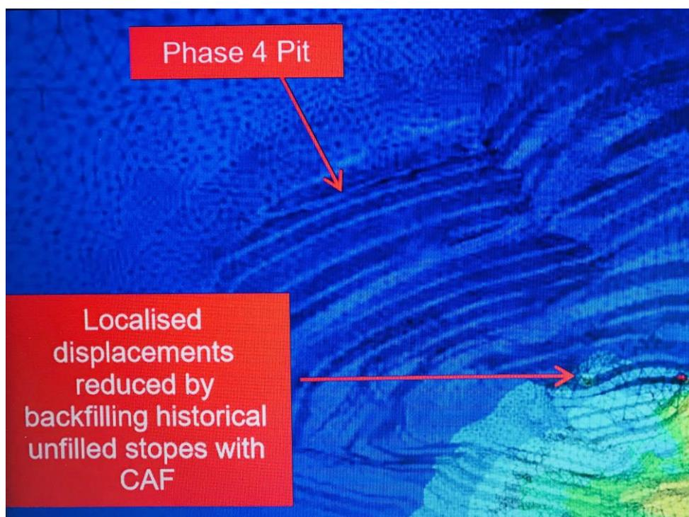
Figure 6. Extract from Figure 42 of AEE Appendix P1 – displacement at base of north wall after completion of MP4 and underground mining with CAF backfill in old stopes below the MP4 base
