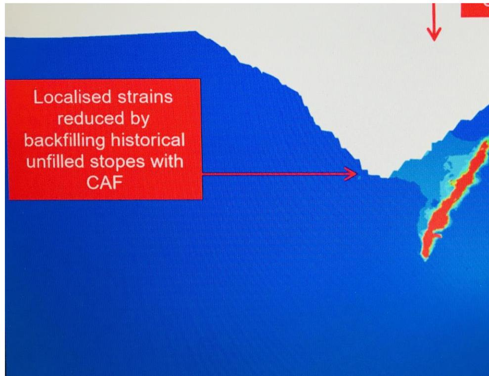
Figure 4. Extract from Figure Appendix G7 of AEE Appendix P1 – shear strain at base of north wall after completion of MP4 and underground mining with CAF backfill in old stopes below the MP4 base
