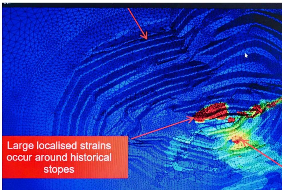
Figure 1. Extract from Figure 24 of AEE Appendix P1 – shear strain at base of north wall after completion of MP4 and underground mining without backfill in old stopes below the MP4 base
