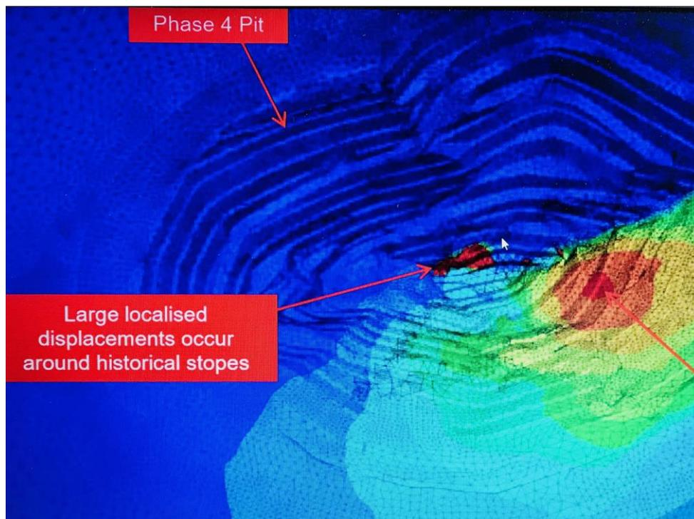
Figure 5. Extract from Figure 18 of AEE Appendix P1 – displacement at base of north wall after completion of MP4 and underground mining without backfill in old stopes below the MP4 base
