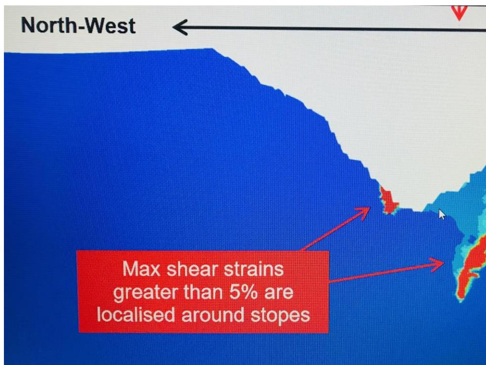
Figure 2. Extract from Figure 25 of AEE Appendix P1 – shear strain at base of north wall after completion of MP4 and underground mining without backfill in old stopes below the MP4 base
