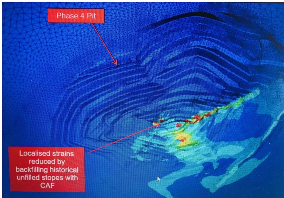
Figure 3. Extract from Figure 43 of AEE Appendix P1 – shear strain at base of north wall after completion of MP4 and underground mining with CAF backfill in old stopes below the MP4 base
