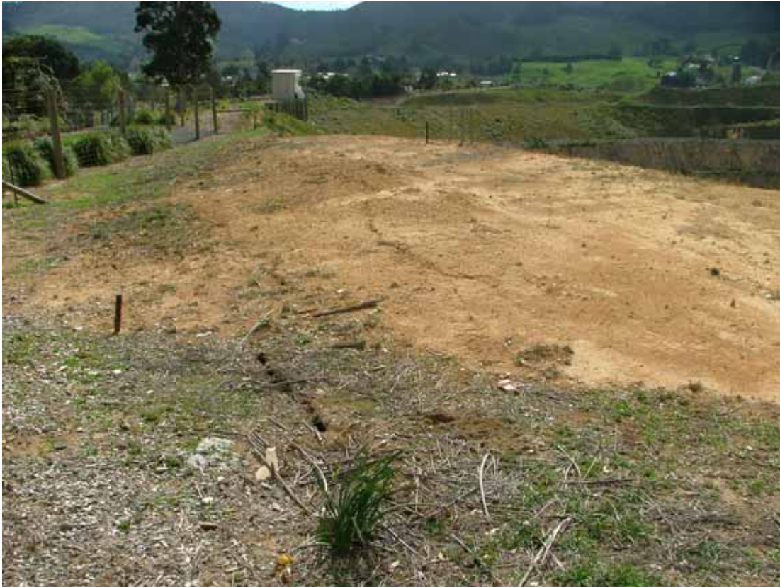
Photo 6 View of surface cracking near the open pit rim which is being monitored with wire extensometers. View looking west.
