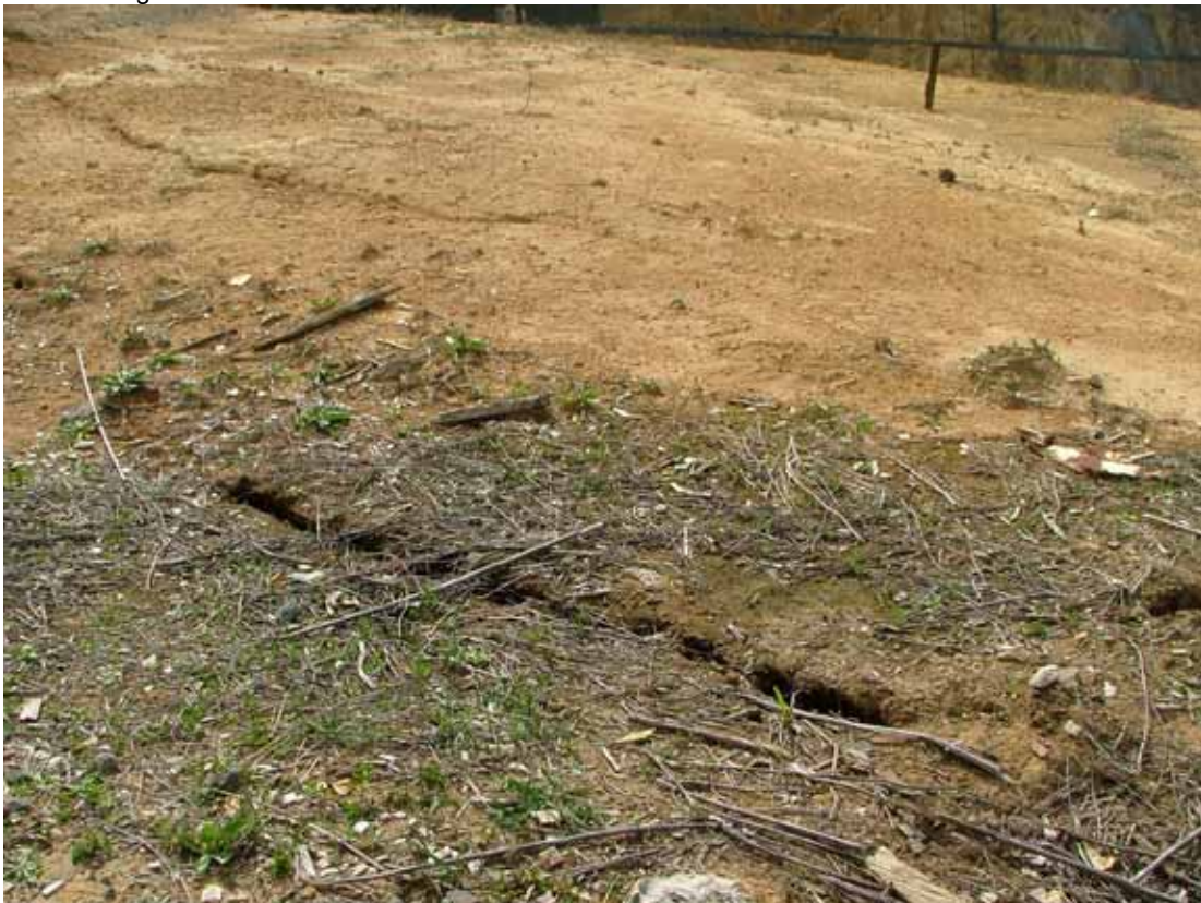
Photo 6 View of surface cracking near the open pit rim which is being monitored with wire extensometers. View looking west.
