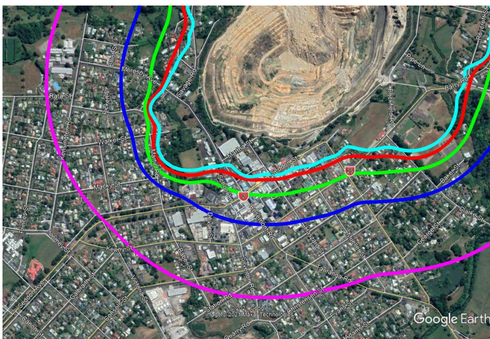
Figure 8 – South west corner of the Expanded Martha Mineral Zone showing the maximum extent of vibration based upon blasting within a reasonably defined pit
