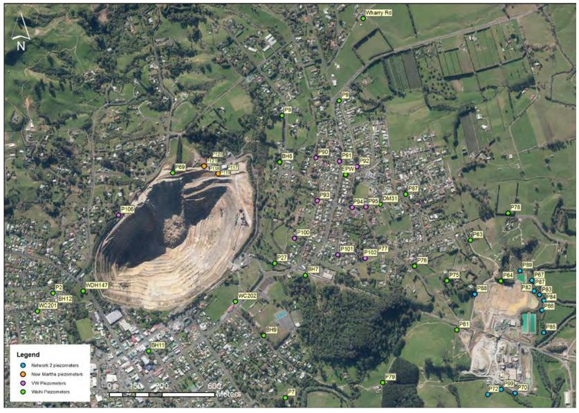
Figure 2: Piezometer Location Plan
