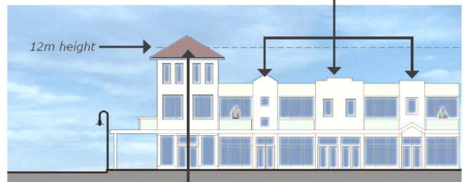
Emphasis provided to corner by three storey element with pitched roof
