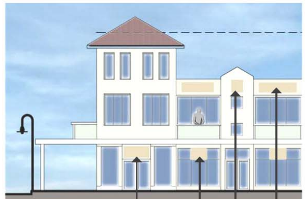
Appropriate locations for signs fitting with building include: above doors; below verandahs; on parapets; and where sign continues pattern of architectural features
