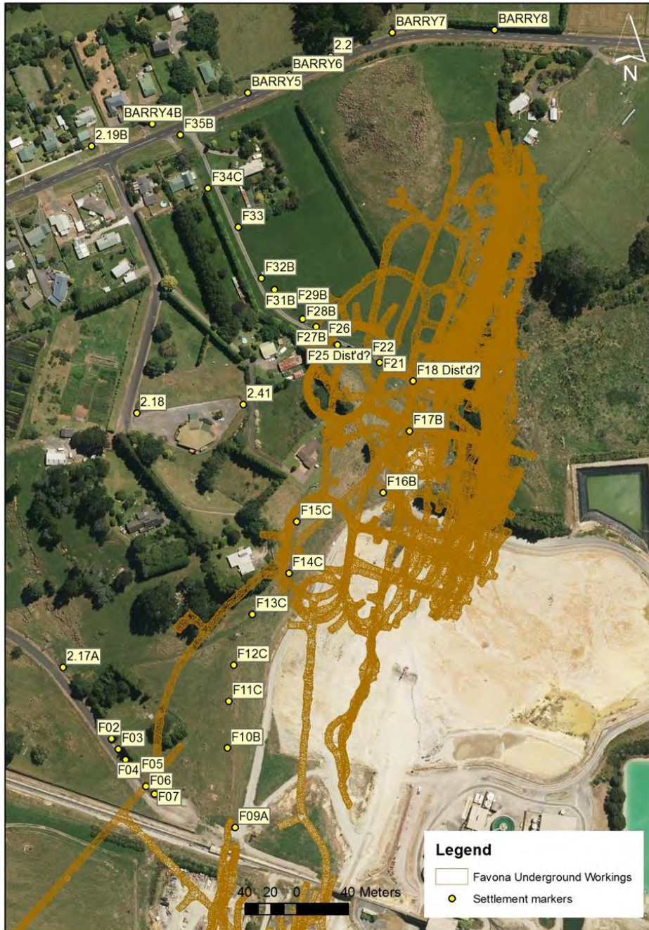
Figure 45: Favona Settlement Markers and Underground Workings
