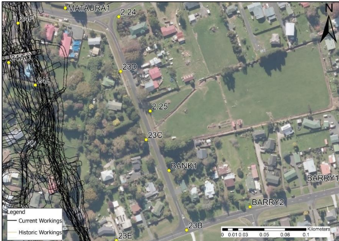
Figure 53. 23C, 2.25 and BANK1 settlement marks and workings.
