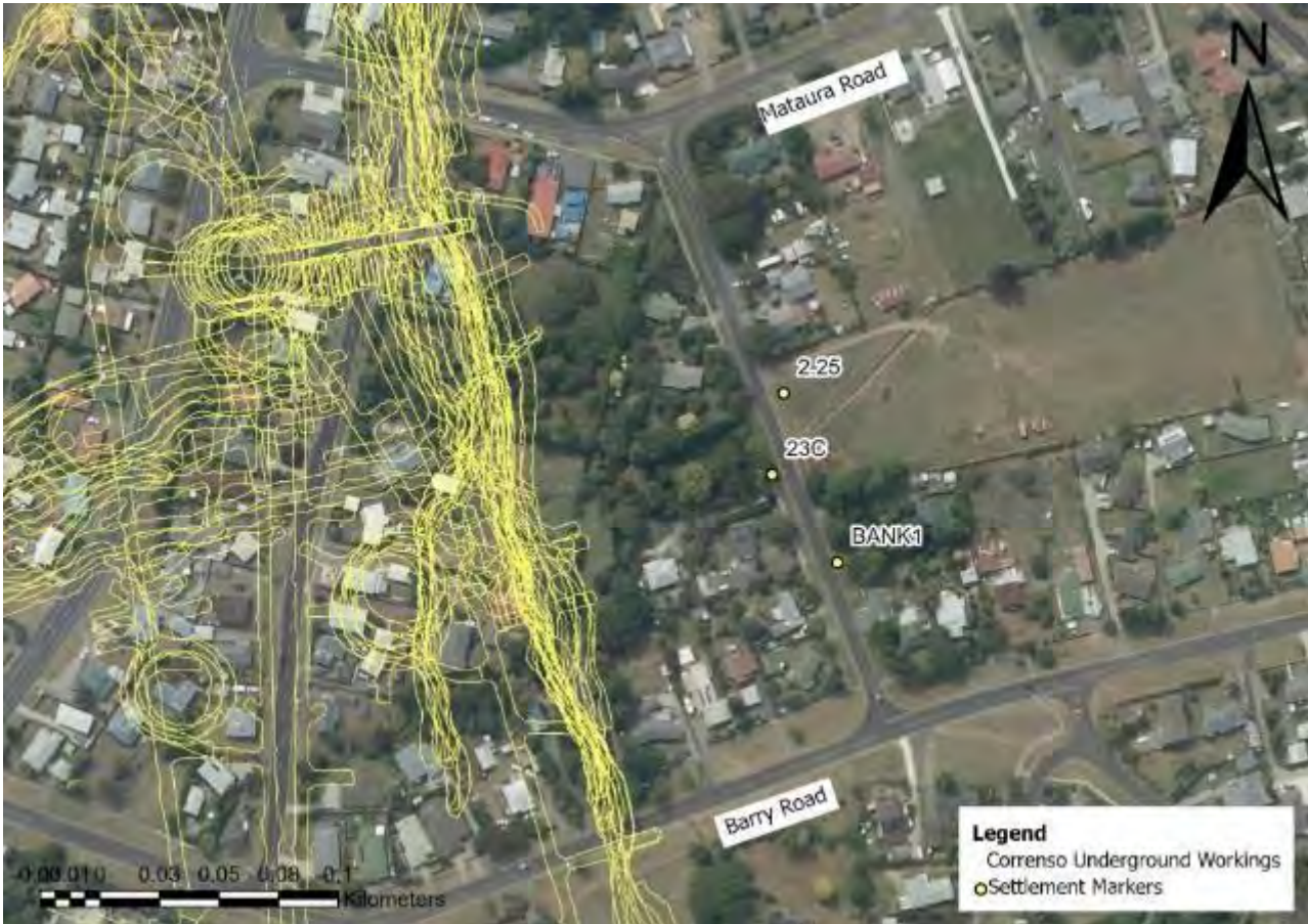
Figure 40: Correnso Tilts and Underground Workings
