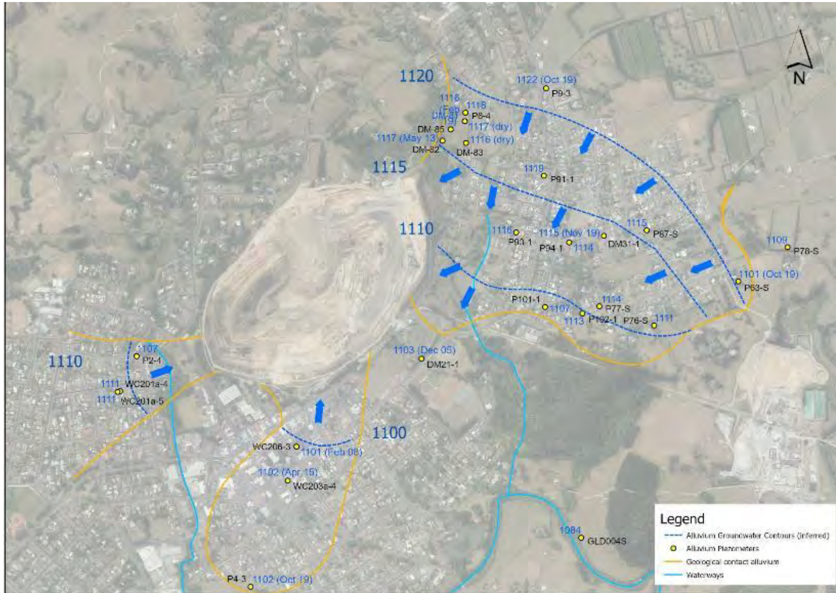
Figure 10: Alluvium water level contours
