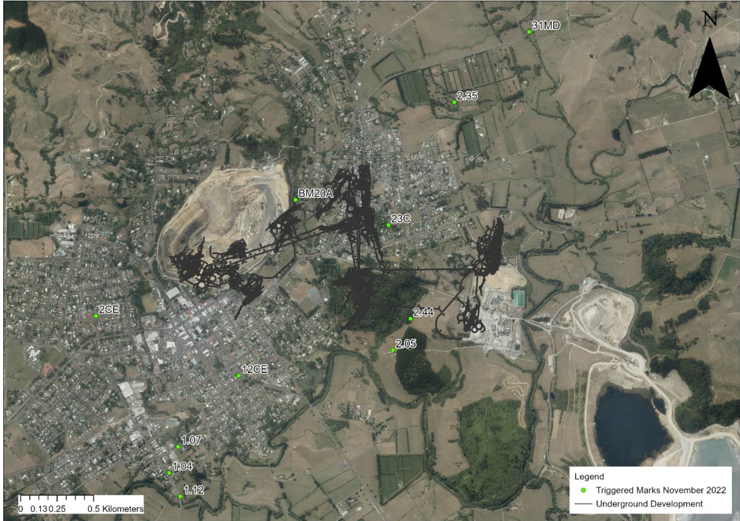
Figure 40: Triggered settlement marks Nov 2022
