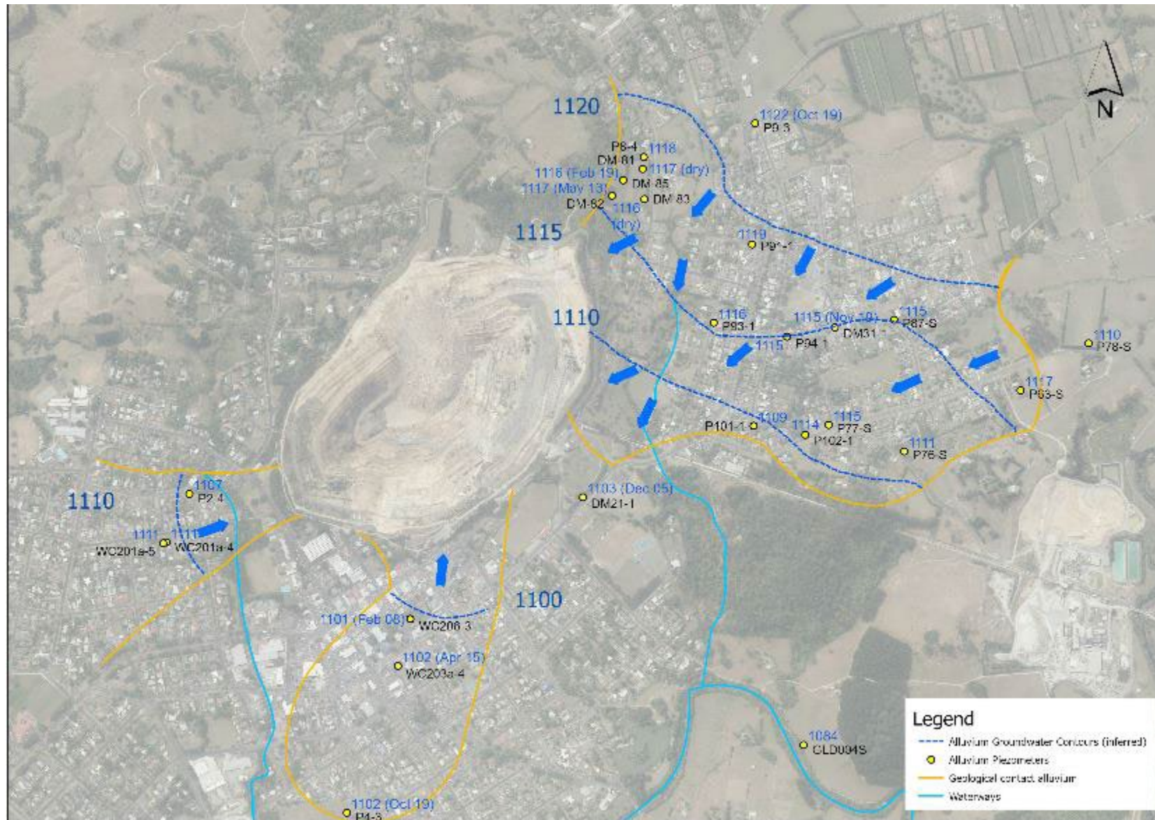
Figure 11. Alluvium water level contours.
