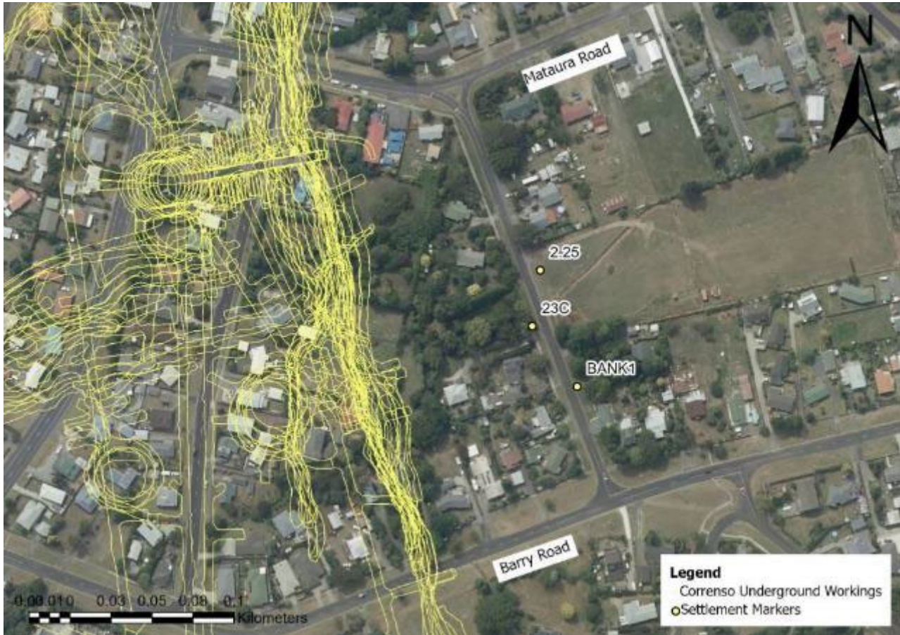
Figure 47: Correnso Tilts and Underground Workings
