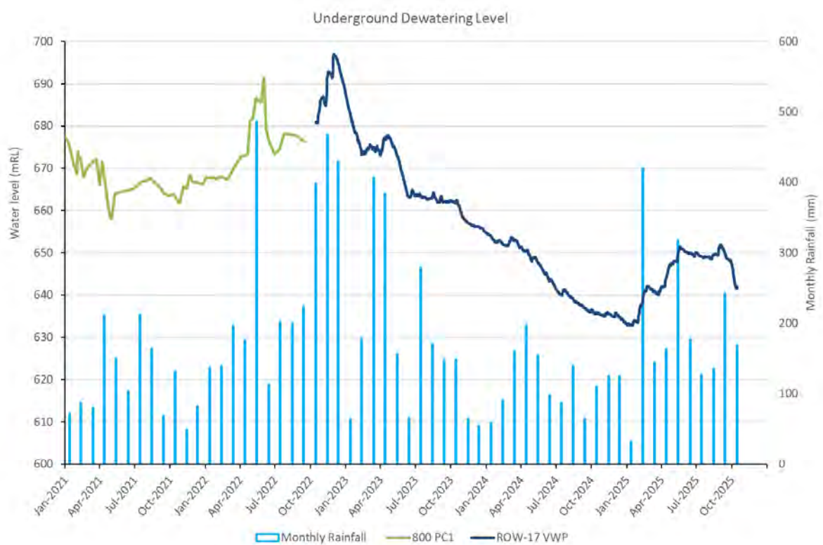
Figure 11. Underground dewatering level
