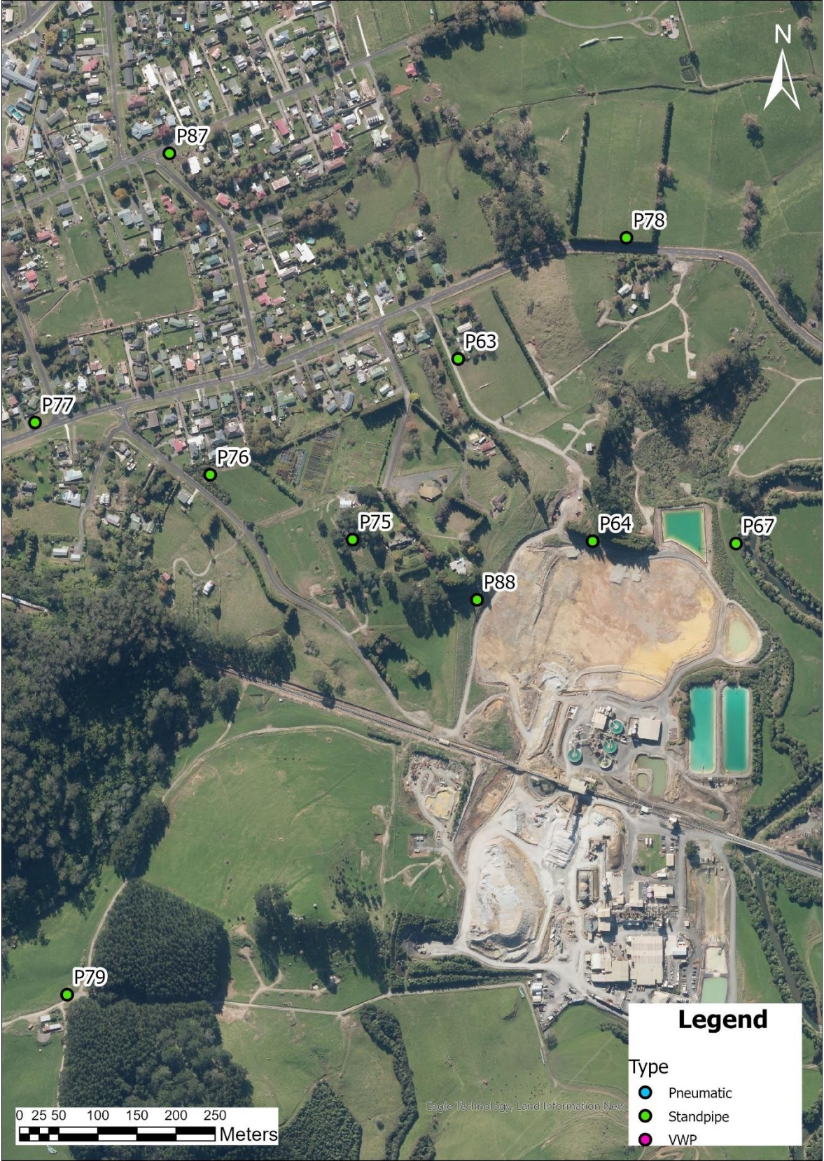
Figure 7: Favona monitoring piezometers
