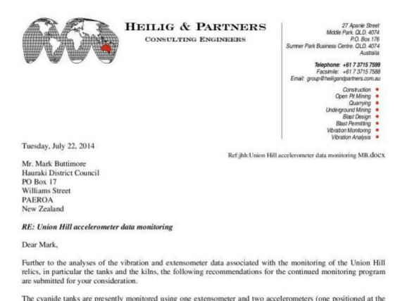
The cyanide tanks are presently monitored using one extensometer and two accelerometers (one positioned at the base and a second at the top of the tank). The kilns are monitored using two extensometers, one positioned across a vertical mortar crack and a second across a horizontal discontinuity. Data from both measurement devices are transferred via modem and analysed to present daily data and trends. In particular, the data are best assessed in terms of the following:
