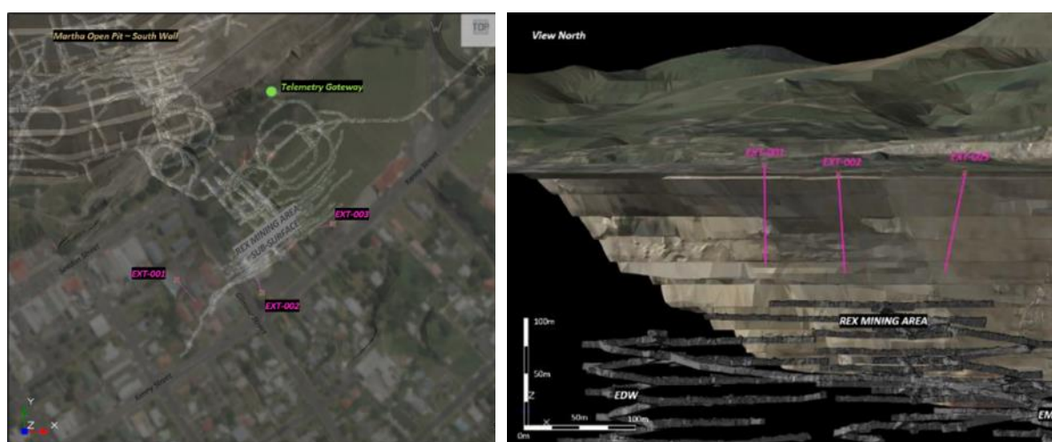
Figure 6: Rex Mining Area Surface Extensometer Locations
