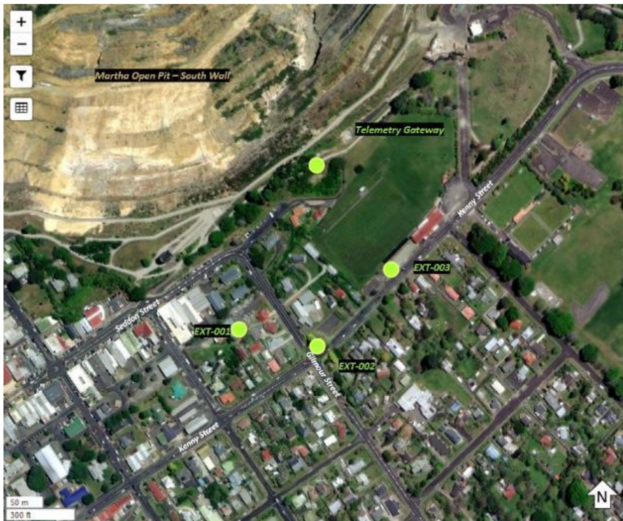
Figure 6: Extensometer Collar Location Plan.
