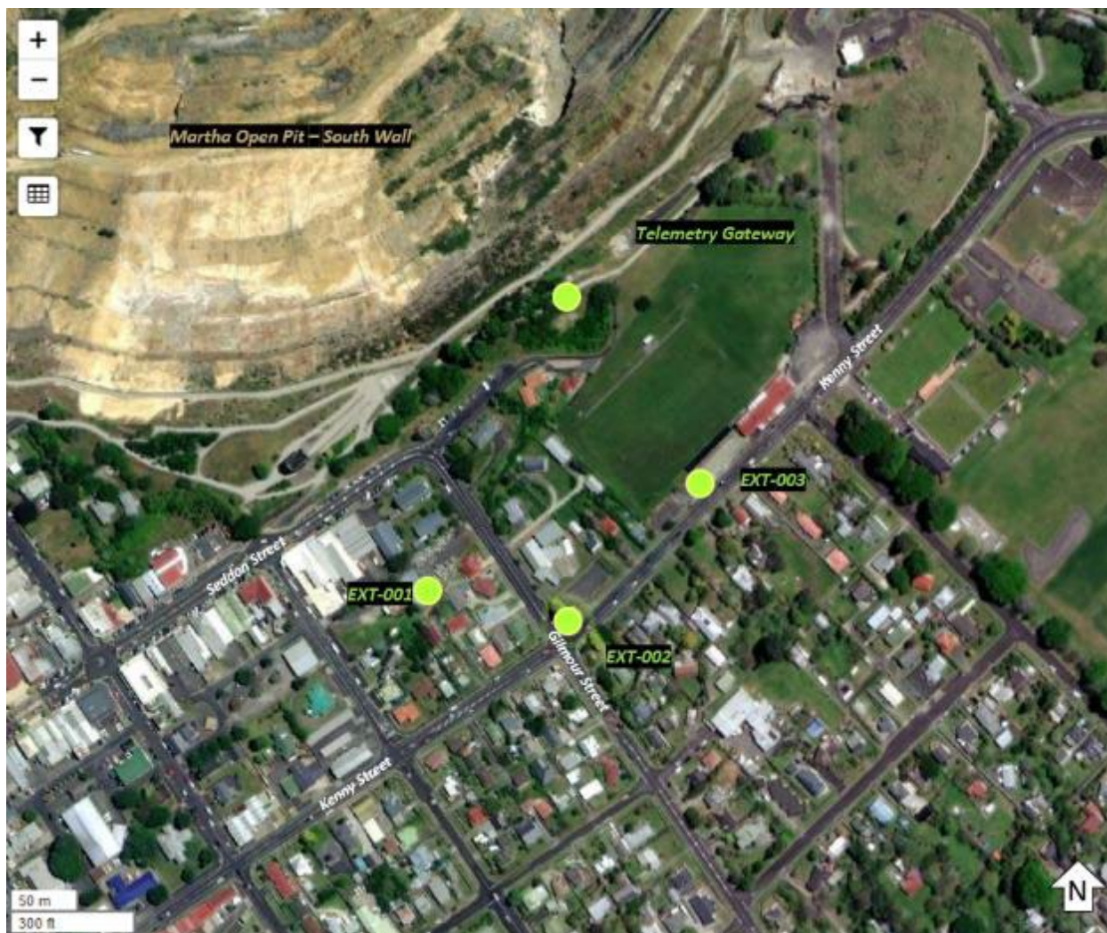
Figure 6: Extensometer Collar Location Plan.
