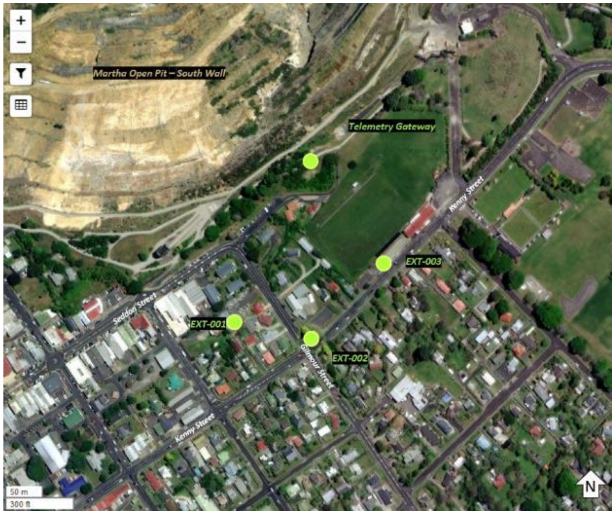
Figure 6: Extensometer Collar Location Plan.
