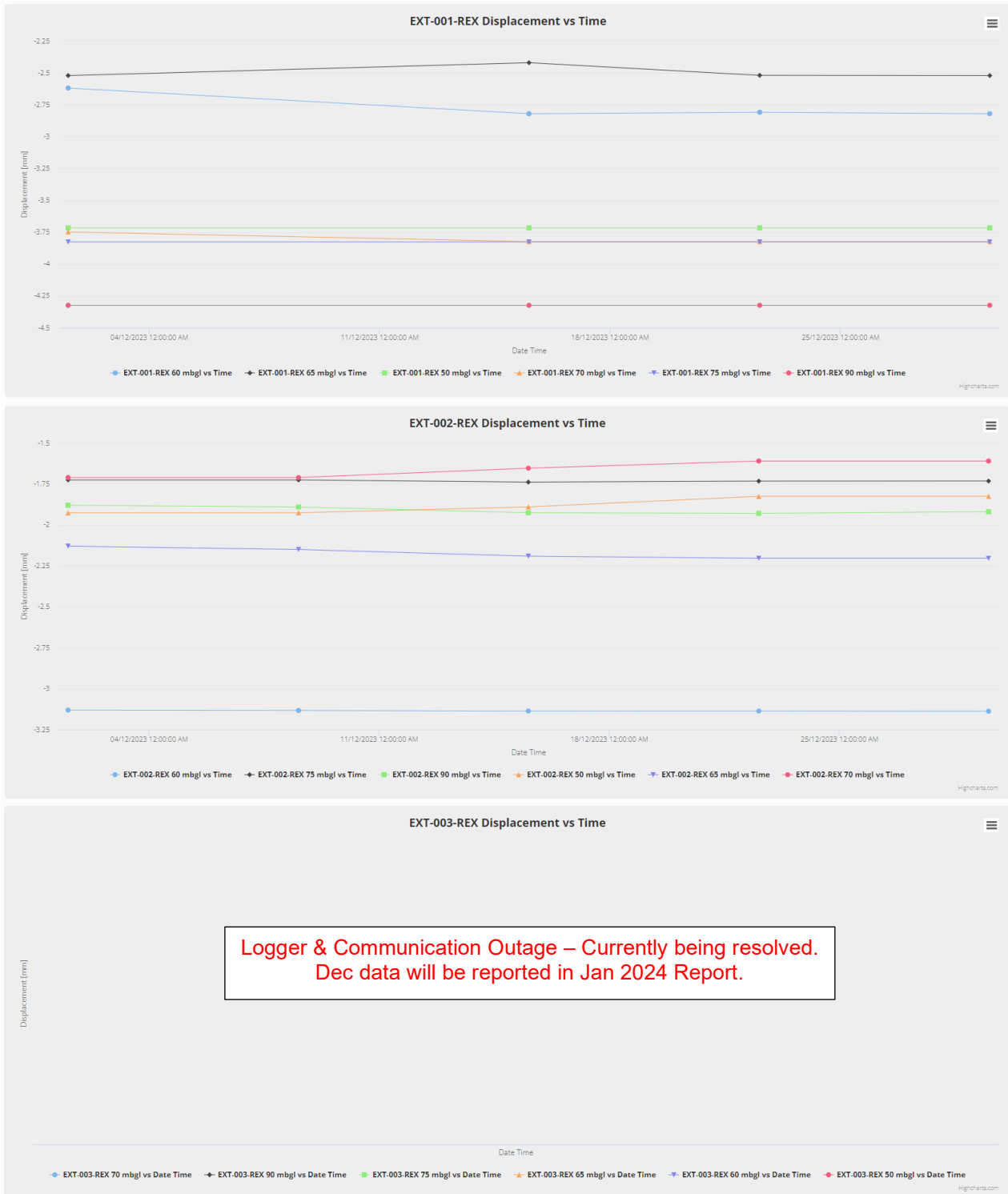
Figure 8: Displacement vs Time for REX Extensometers – December 2023.
