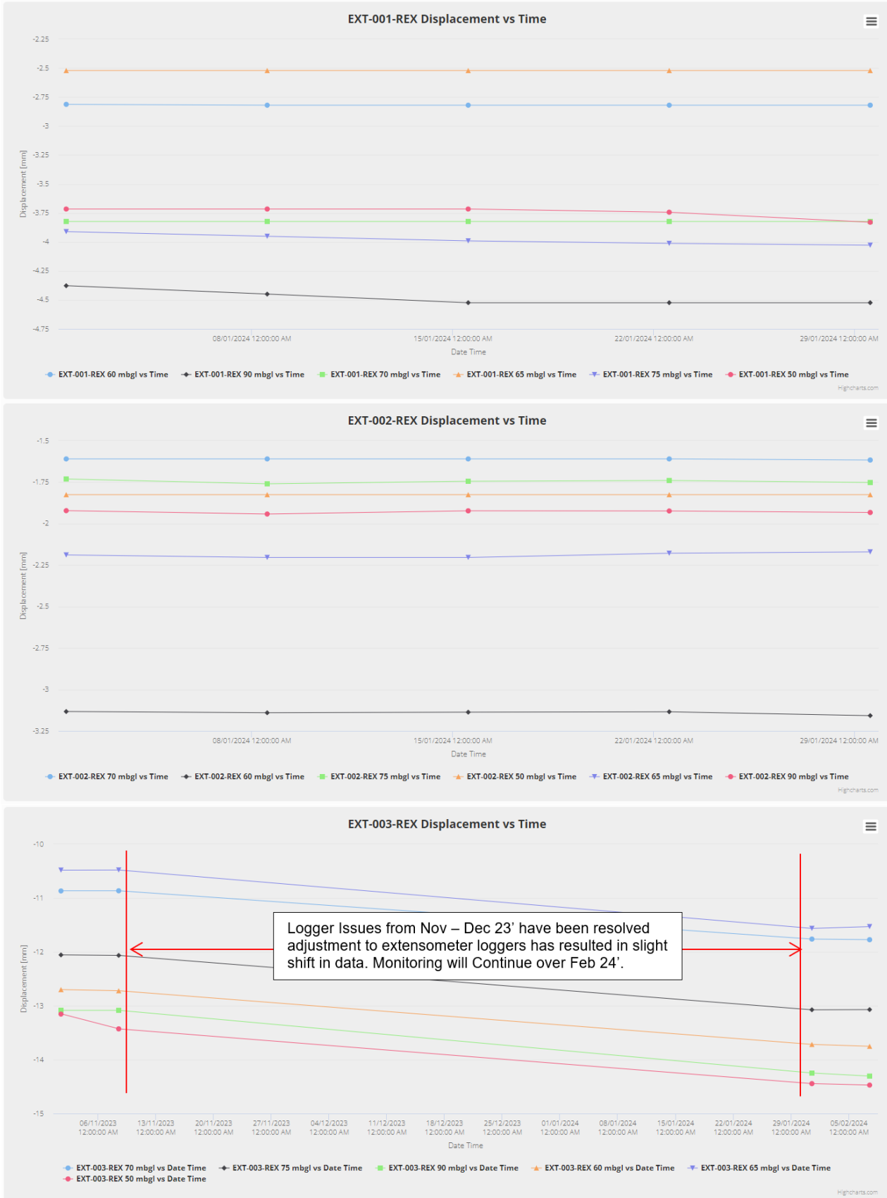
Figure 9: Displacement vs Time for REX Extensometers – January 2024.
