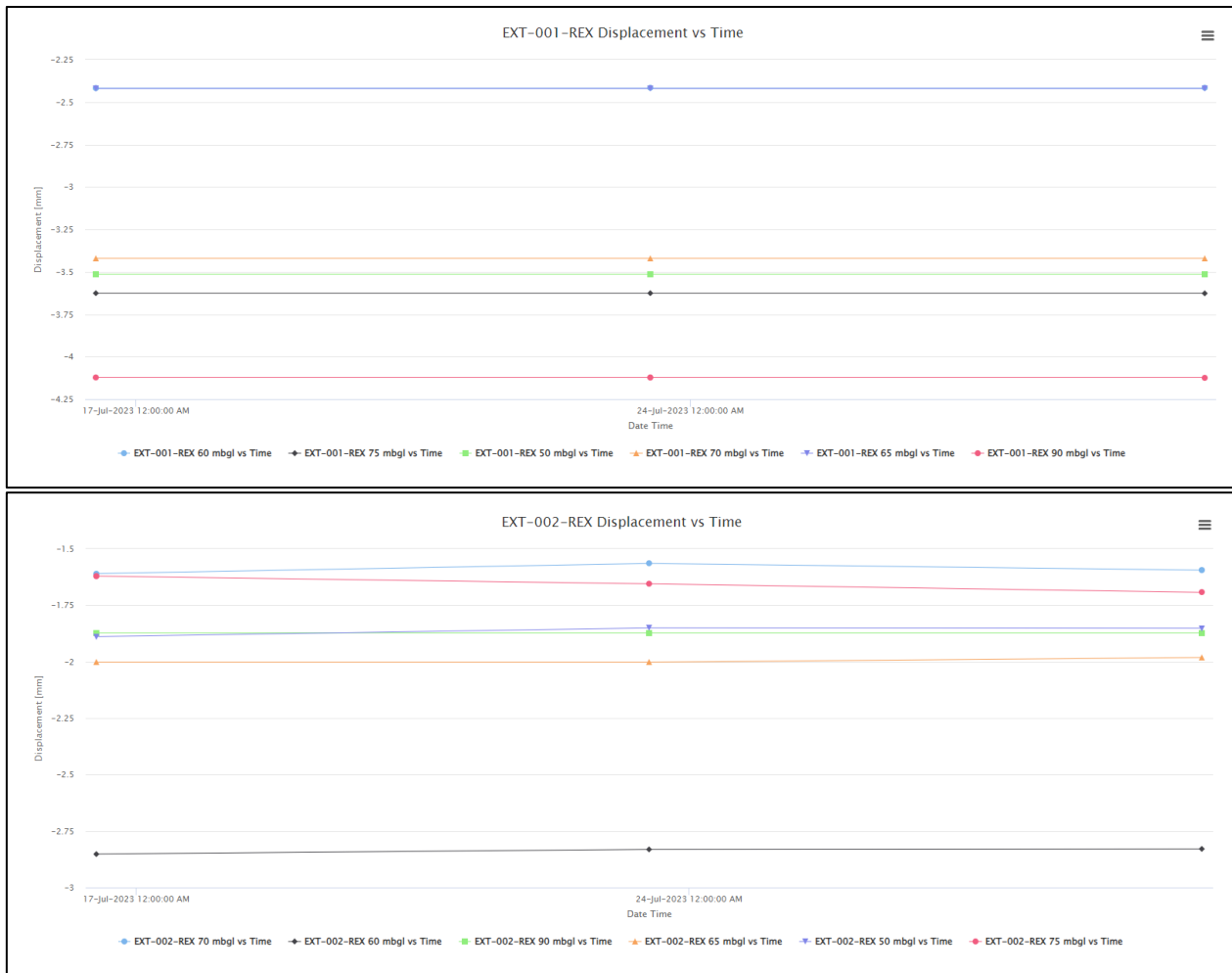
Figure 9 – Displacement vs Time for REX Extensometers – July 2023
