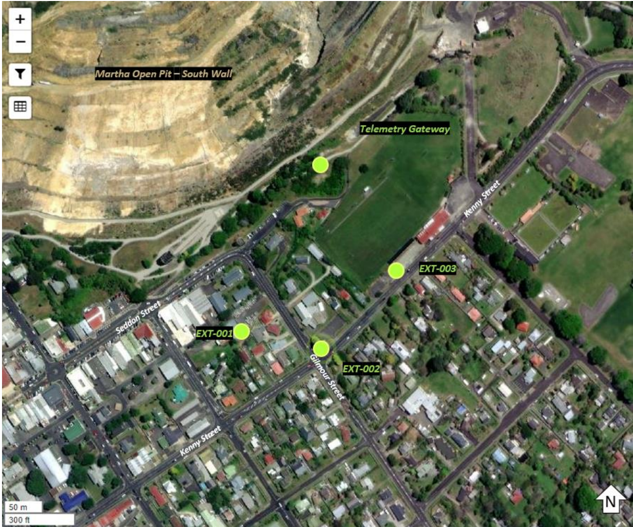
Figure 6: Extensometer Collar Location Plan
