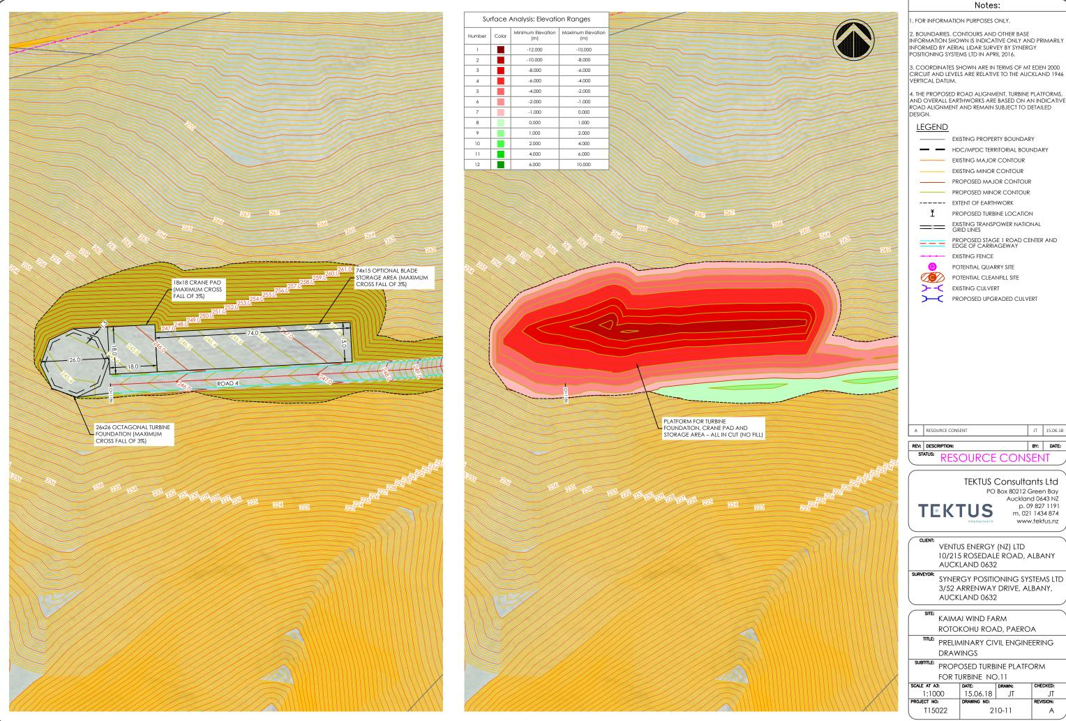
2. BOUNDARIES, CONTOURS AND OTHER BASE INFORMATION SHOWN IS INDICATIVE ONLY AND PRIMARILY INFORMED BY AERIAL LIDAR SURVEY BY SYNERGY
