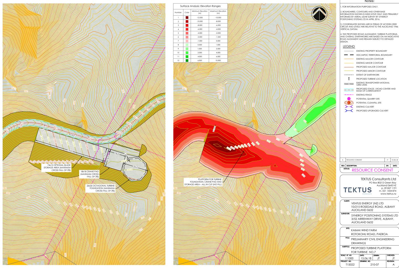
2. BOUNDARIES, CONTOURS AND OTHER BASE INFORMATION SHOWN IS INDICATIVE ONLY AND PRIMARILY INFORMED BY AERIAL LIDAR SURVEY BY SYNERGY POSITIONING SYSTEMS LTD IN APRIL 2016.
