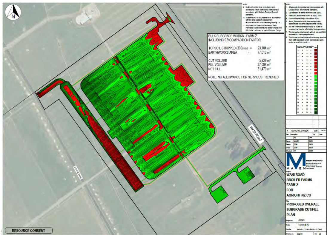
Figure 5: Earthworks cut and fill plan – Farm 2
