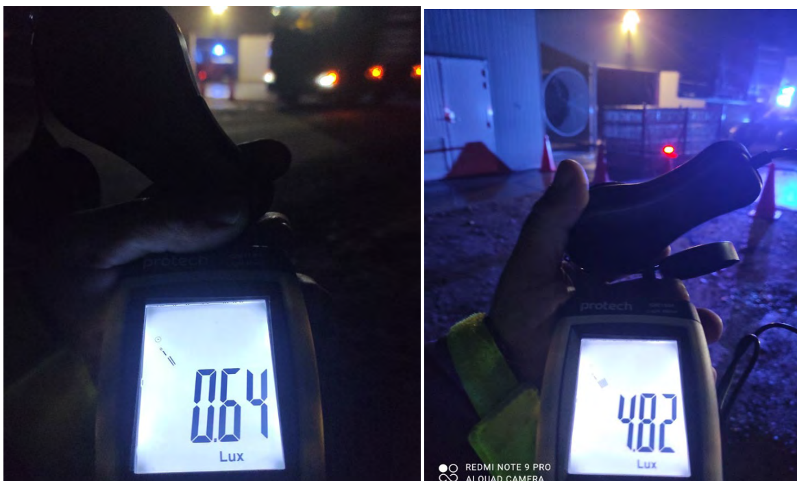
Figure 2: Photos showing lux measurements (Left: Lux reading within the lit area. Right: Lux reading approximately 15m away from lit area)
